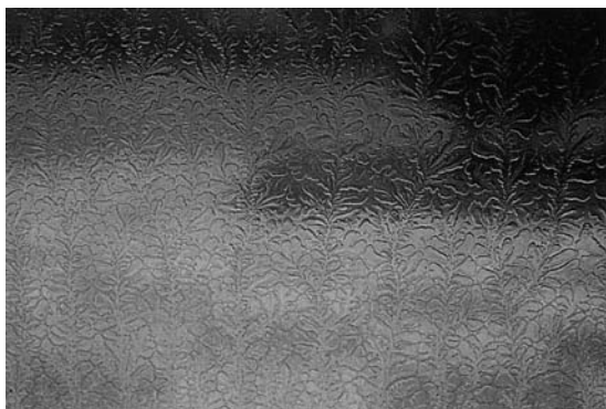
Fig. 2.11: Viscous fingering patterns in the layered window pane of the Hotel Los Lobreros in Seville. These patterns are formed as air penetrates into the plastic film between the glass planes. (Photo: Juan Manuel Garcia-Ruiz, University of Granada.)
