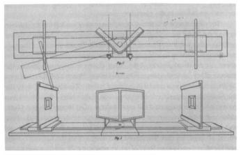
Diagram of the operation of the Wheatstone stereoscope.
