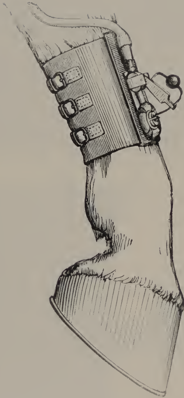
11. Leather bracelet for the inscription of the horse's gait, 1872. Animal Mechanism .
