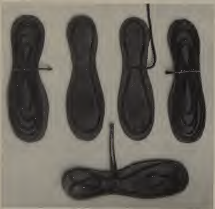
55. Odographic-dynamographic shoes, 1883–84: (A) Air capsule and spring in the heel. (B) soles with rubber tubing. Collège de France.
