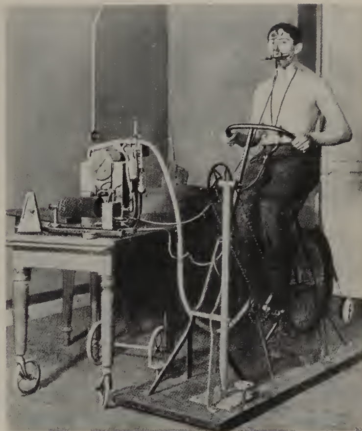
178. Jules Amar, subject using dynamometric bicycle and spirometer, 1912. The Physiology of Industrial Organisation and the Re-employment of the Disabled (London, 1918).
