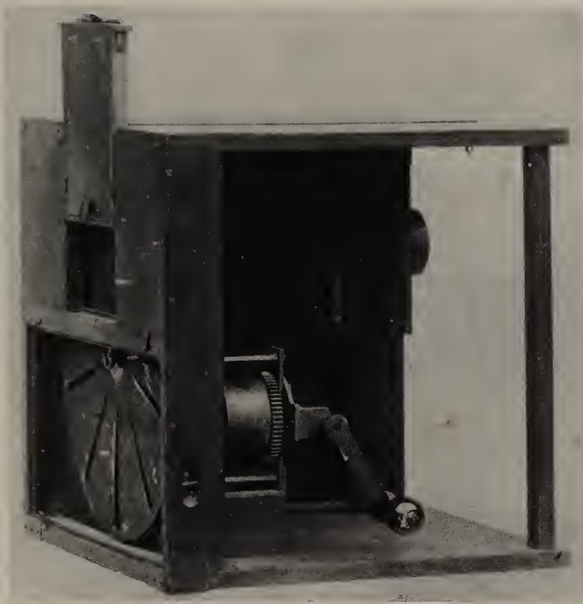
32. Marey's first fixed-plate chronophotographic camera, third version with ten slots in the disk shutter, 1882. Beaune.
