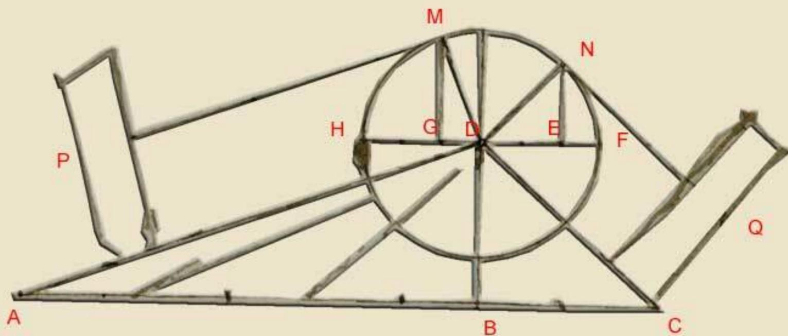
Weight Q, because of the right angle N above DF at point E, weighs  $\frac{2}{3}$  of its initial weight, which was 3 pounds. Its force therefore remains 2 pounds. Weight P, also 3 pounds, has a potential force of one pound because of the right angle M located at point G on line HD. Therefore we have here one pound against 2 pounds.
