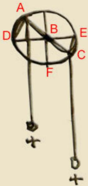
If it were possible to suspend the balance in the center of its gravity, it would stay still and never oscillate, in whatever slanted position it was situated, as is seen in a round balance.
