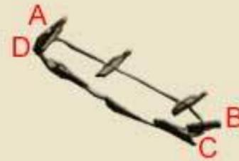
The palm of the hand goes from point A to point B, always at the same angle, descending and putting pressure on the air. When it reaches point B, it immediately flattens and turns back, following the line CD, and having arrived at D, it quickly turns around and goes descending by the line AB, and in turning always turns around the center of its width.
