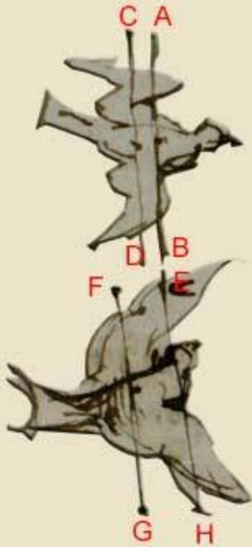
*When the bird wants to rise, its center of gravity remains behind its center of resistance. As if the center of gravity just cited was situated at FG and the center of resistance at EH.*
