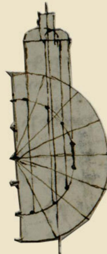
The center of gravity of pyramids of two equidistant sides lies in the third point along of its length toward the base. And if you wished to find the exact center of gravity of the semicircle, divide it into so many triangles so that the curvature of their bases almost seems a straight line, and then you have the example illustrated here above, and you will find the position of the center almost perfectly.
