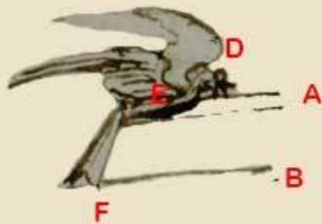
When the bird is above the wind and turning its beak and breast into the wind, then the bird could be overturned by such a wind, unless it lowers its tail so that not much wind strikes it; and in so doing, it is impossible to be overturned. This can be proved by the first principle of the "Elements of Machinery", which demonstrates how things in balance, which are struck beyond the center of their gravity, tilt down their opposite parts below that center of gravity.
