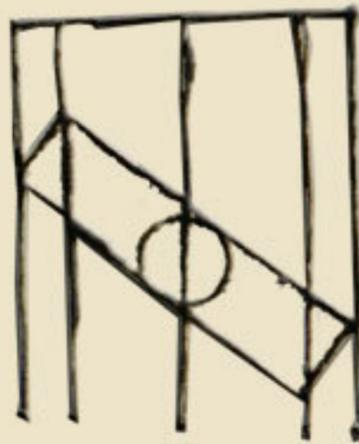
This case shows that even though the perpendicular weights are equal, the oscillation of the balance is not caused by this--on the contrary, this would hinder its movement. Nor is it caused by the reasons illustrated in the fifth scale shown above, but by looking at the seventh scale, the cause proves to be physical movement.
