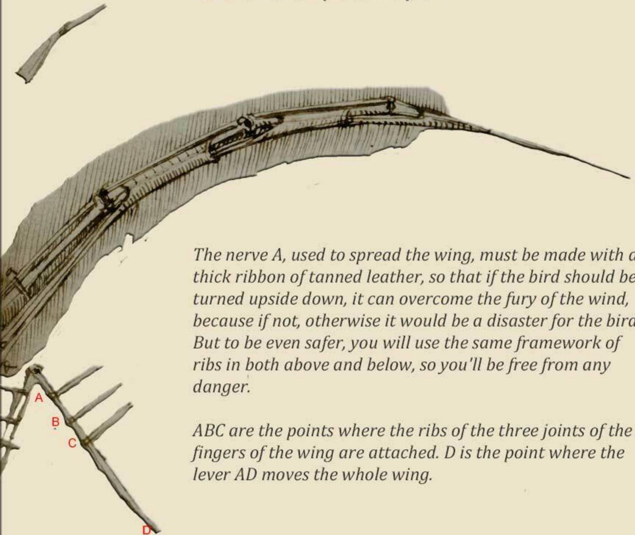
The nerve A, used to spread the wing, must be made with a thick ribbon of tanned leather, so that if the bird should be turned upside down, it can overcome the fury of the wind, because if not, otherwise it would be a disaster for the bird. But to be even safer, you will use the same framework of ribs in both above and below, so you'll be free from any danger.
