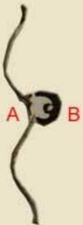
*Then, when the bird is in position AB, as A is lighter than the place where the "engine" B is located, the lighter point A will always be above the heavier point B, so it will never happen that A is in front of B, except in case of accidents and for a very short time.*
