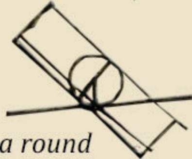
In a round or circular balance, oscillation does not occur because its parts always move equally around the fulcrum.
