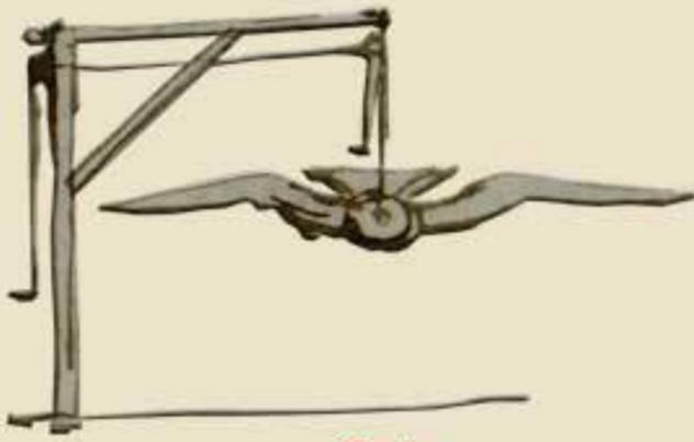
*This is done to find the bird's center of gravity; without this equipment the bird as built would be of little use.*
