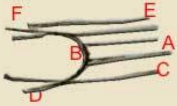
(continued from folio 10R) ...on its upper surface, the force of the wind, which strikes from above, is not at its full force, because part of the wind, like a wedge, strikes the underside of the wing. The wind divides at the bottom near the middle point of the edge of the humerus, raising the wing up almost with the same force as the wind that strikes the upper surface of the wing and pushes it downward.
