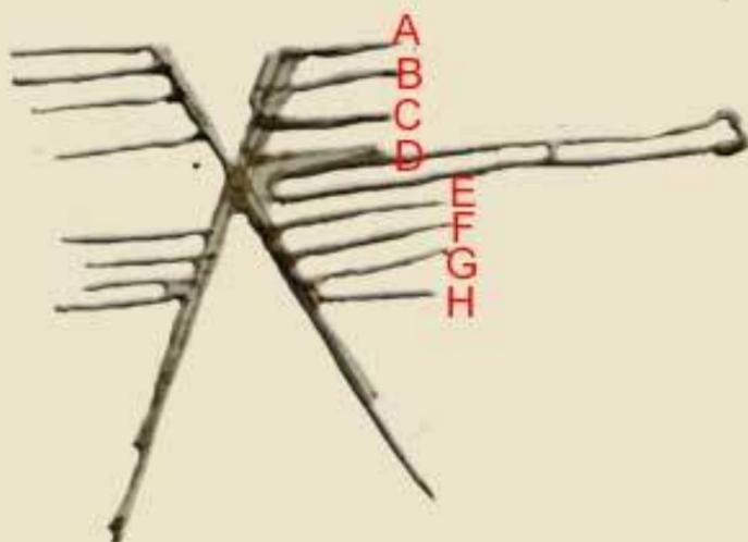
ABCD are the four upper ribs that serve to raise the wing and are as strong as the ribs below EFGH. In the event of the overturning of the bird, both the upper and lower ribs will be of use, even though a single, thick, wide rib of treated leather might be enough. To check what I have said we will make some more practical tests.
