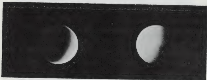
Fig. 75. — A concave hemispherical cup on the left and a convex hemisphere on the right lighted by a light-source of large angle such as a window.
