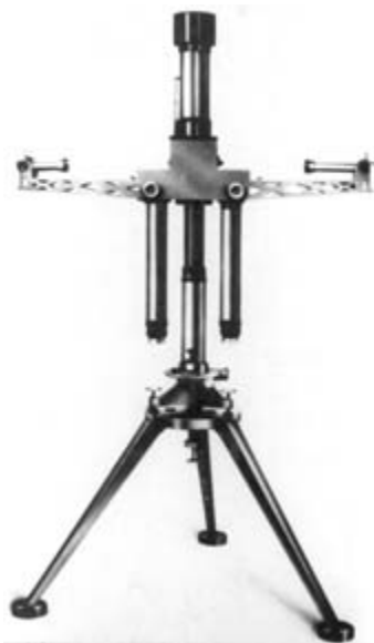
A torsion balance used by Eötvös' assistant and successor Dezső Pekár in the 1930s to make measurements of variations in the earth's gravity. The armature rotates around the vertical axis.
